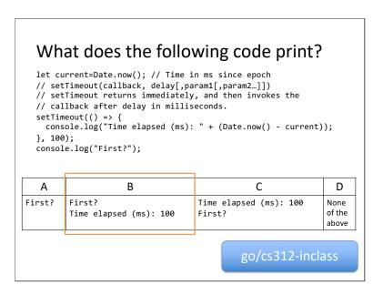
Context: setTimeout returns immediately, and then invokes the callback after delay in milliseconds.
