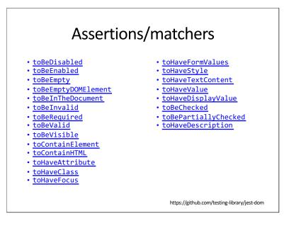
Once we have the DOM element, we need to make an assertion. The testing library provides some custom matchers in the jest-dom package (an extension to Jest that adds matchers (assertions) relevant to the UI). In our previous example, we could use the toBeDisabled matcher to assert the button is disabled until we check the box to agree to the terms and conditions. To do the latter we will need a way to simulate the user interaction.
